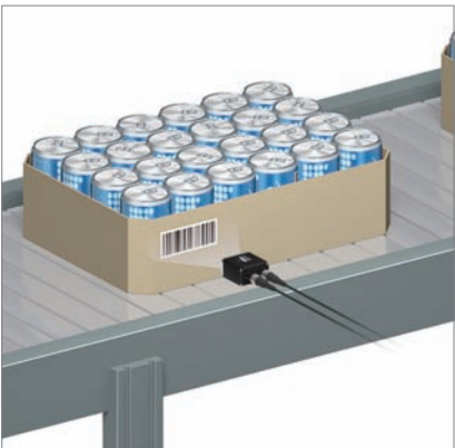
Code print quality verification of packing boxes
