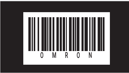
Insufficient quiet zone
